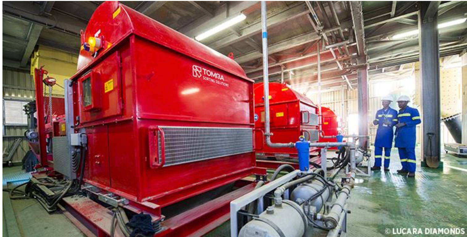
Tomra large diamond recovery (LDR) machine using XRT sensors at Karowe Mine, Botswana.
